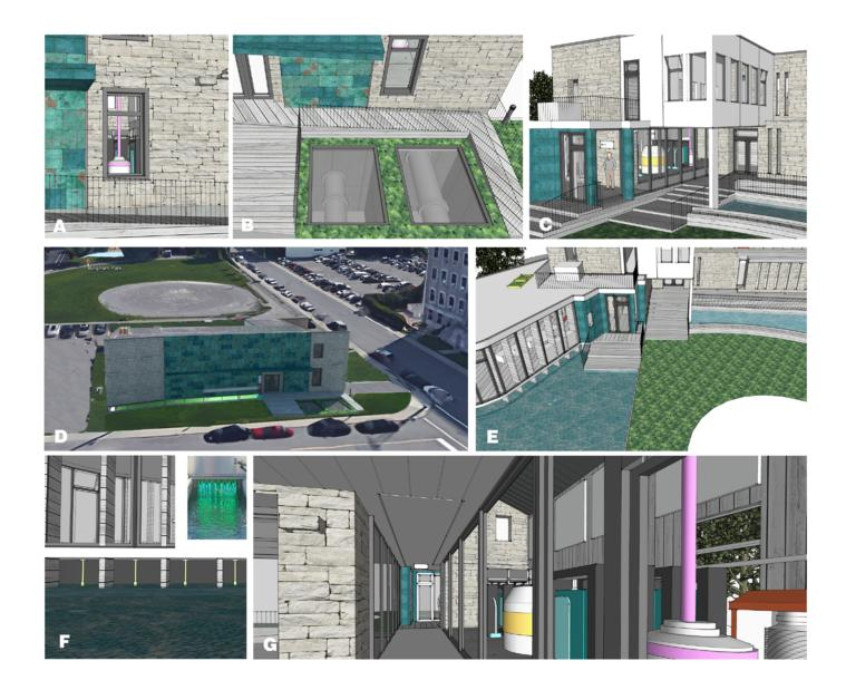
Figure 46: A: Selective views into interior equipment. B: Major sewer infrastructure leading in and out of facility is revealed. C: Exterior views to treatment space. D: Interior lighting at grade. E: Treated effluent pool vs. City water supply pool. F: UV treatment detail. G: Interior views along treatment space with room for educational posters above.
