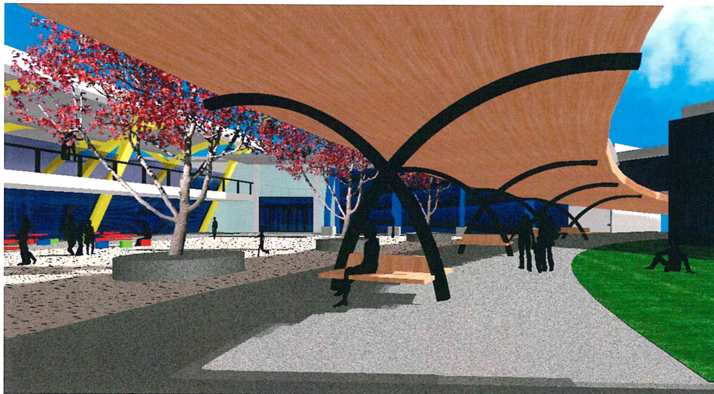
STREET ROOF STEEL FRAMES ARE ROTATED TO CREATE SUPPORT FOR SEATING
