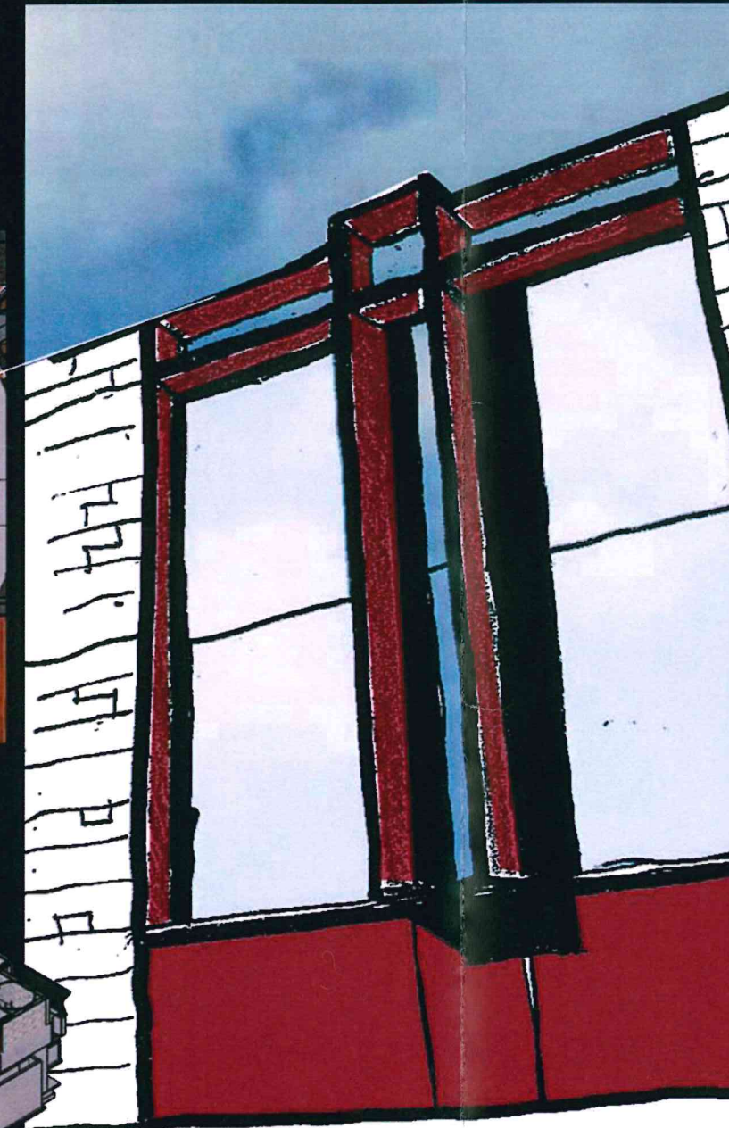
RENDERING SHOWING BACK SPA WINDOW, STEEL MULLIONS, FROSTED GLASS AND CLEAR GLASS PANELS
